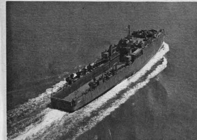
High deck forward shelters crew of LSD on long ocean crossings or in heavy weather. Block superstructure forward, two small stacks port and starboard, deck well help identify type.
